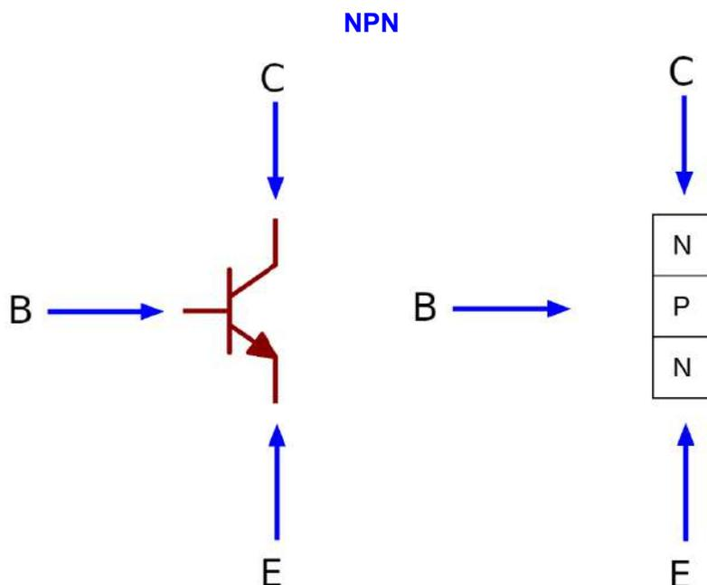
The NPN Type consists of two N-Regions separated by a P-Region, so we can suppose a diode between B - C and between B - E.
