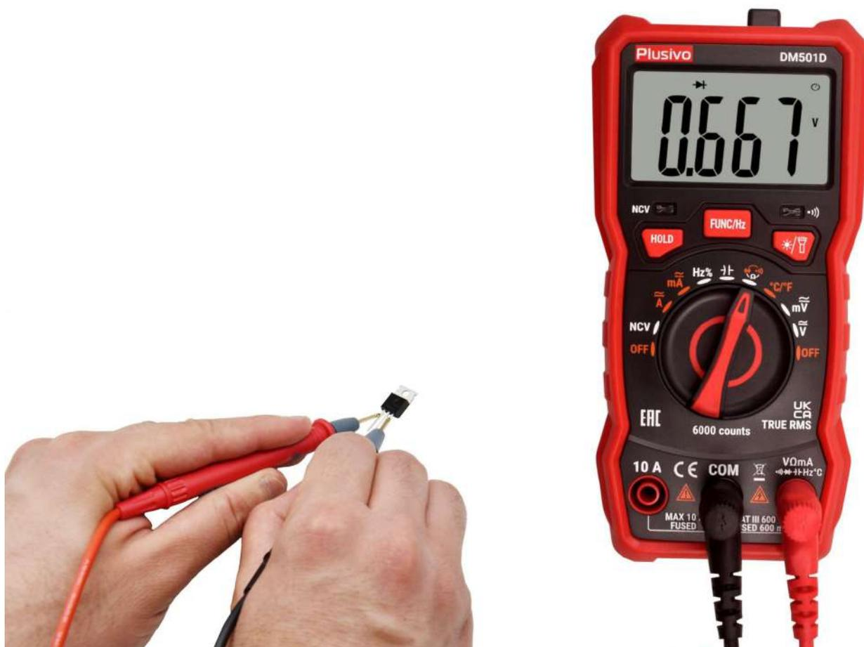
The measured forward voltage in this figure is 0.667 V.
