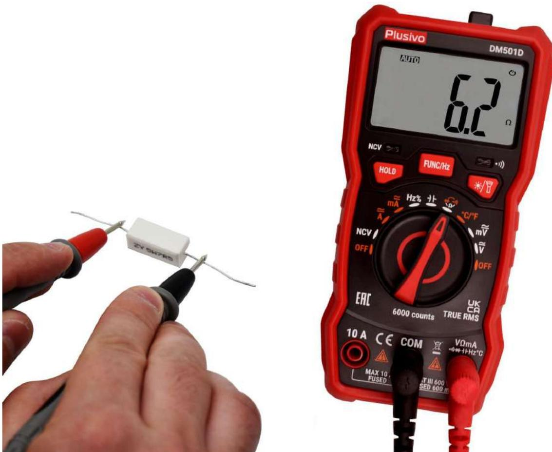
The resistance measured in this figure is 6.2 Ω
