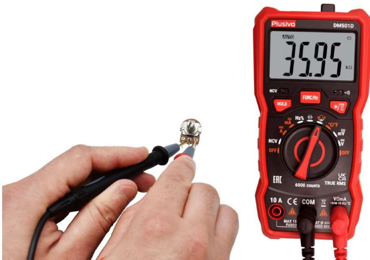
The measured resistance in this figure is 35.95 kΩ.
