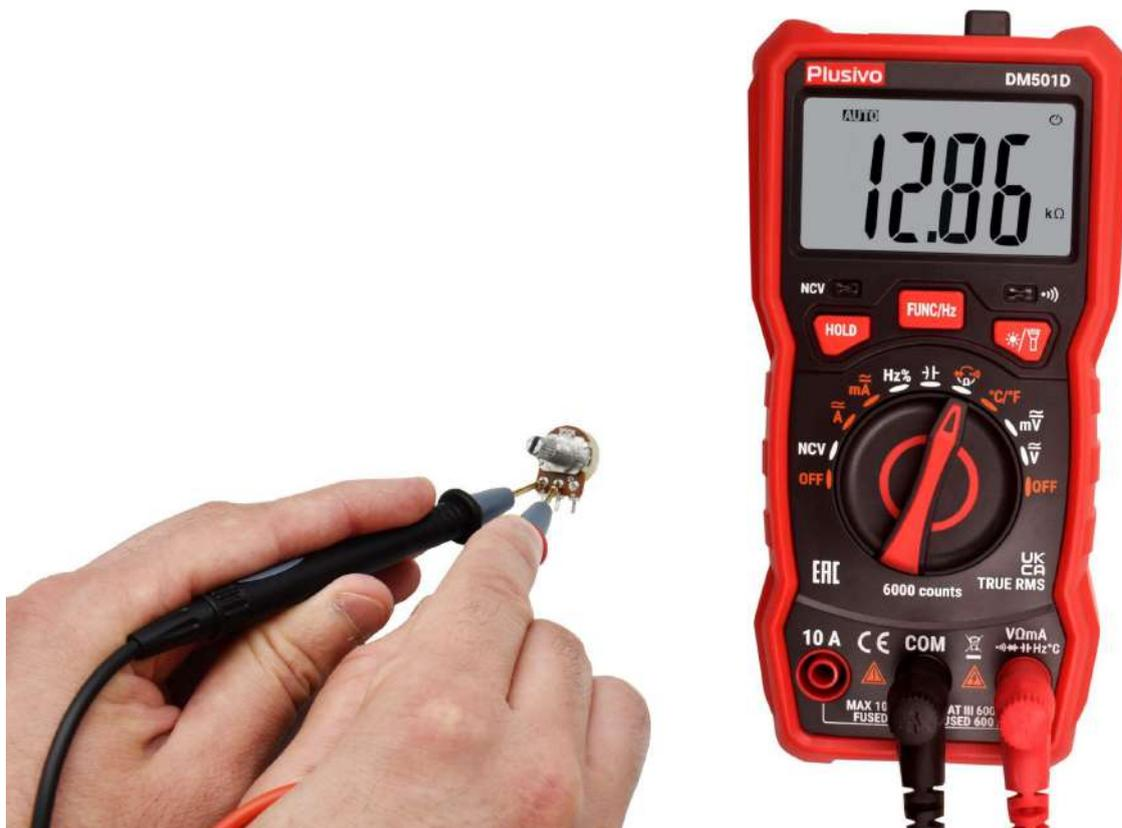
The measured resistance in this figure is 12.86 kΩ.
