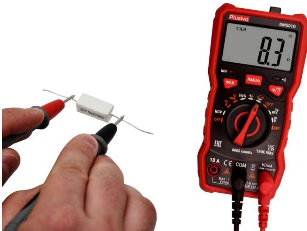
The measured resistance in this figure is 8.3 Ω.
