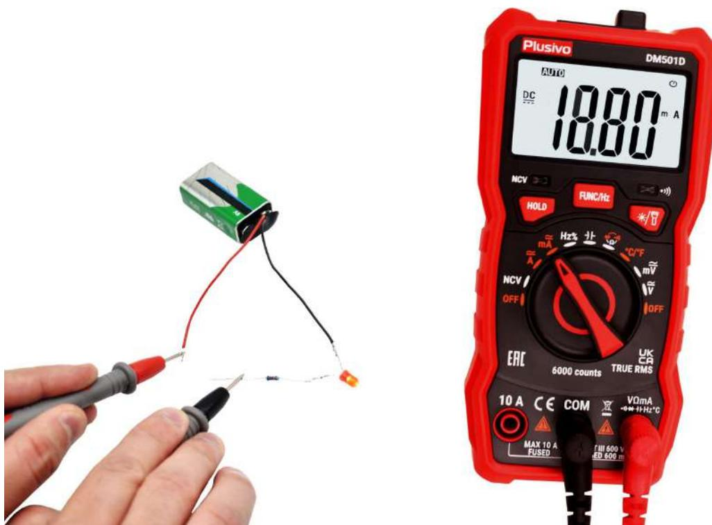
The measured current in this figure is 18.80 mA.
