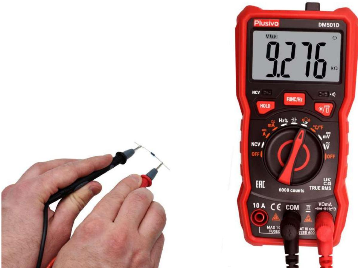
The resistance measured in this figure is 9.276 k $\Omega$
