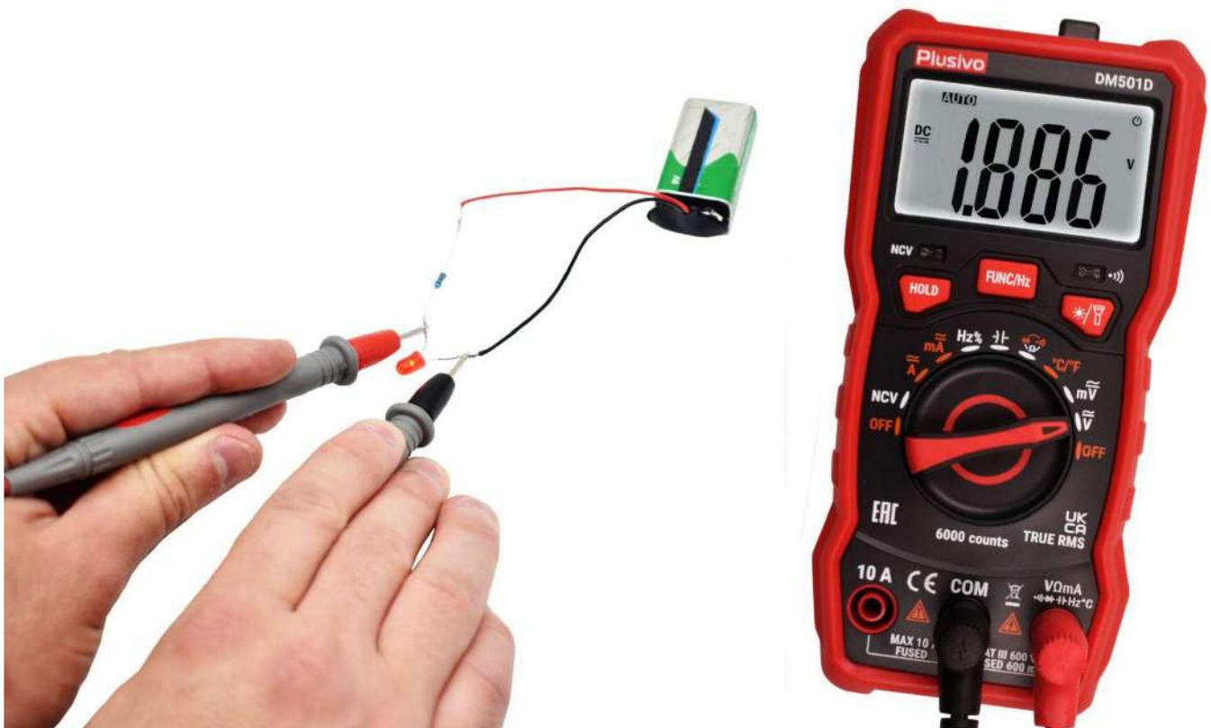
The measured voltage in this figure is 1.886 V DC
