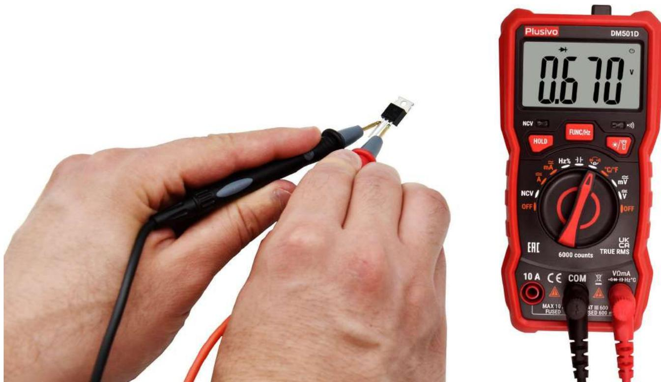
The measured forward voltage in this figure is 0.670 V.
