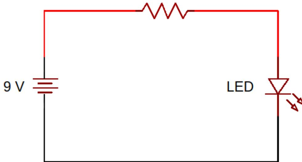
Now, we need to build the circuit with a red LED, and we will use a high resistor, in our case, we will use a **2.2 k $\Omega$**  resistor and measure the forward voltage using the multimeter.
