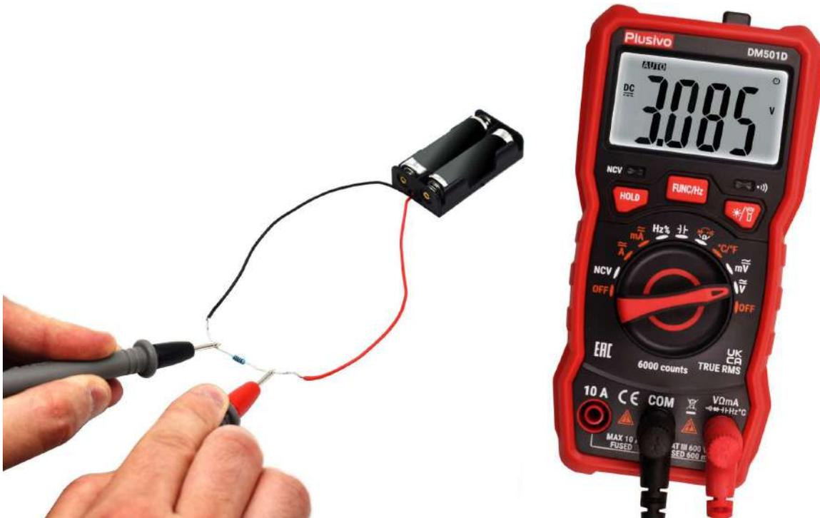
The measured voltage in this figure is 3.085 V DC.
