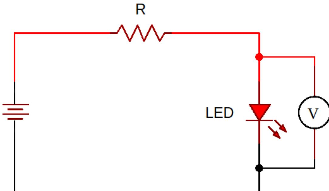
To measure the forward voltage we connect a high value resistor, so we ensure that a low current will pass through the LED.
