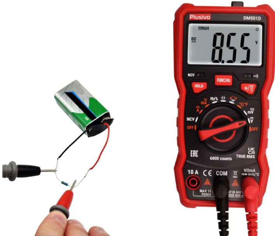
The measured voltage in this figure is 8.55 V DC.
