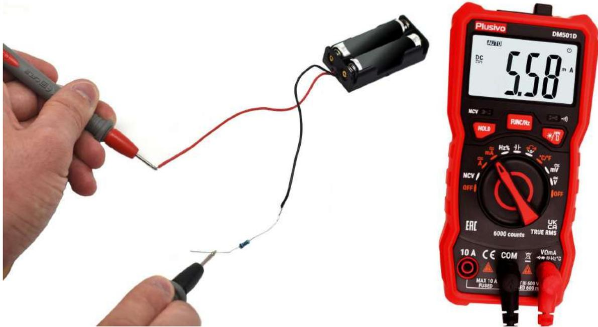
The measured current in this figure is 5.58 mA
