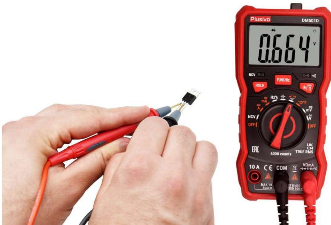
The measured forward voltage is 0.664 V.
