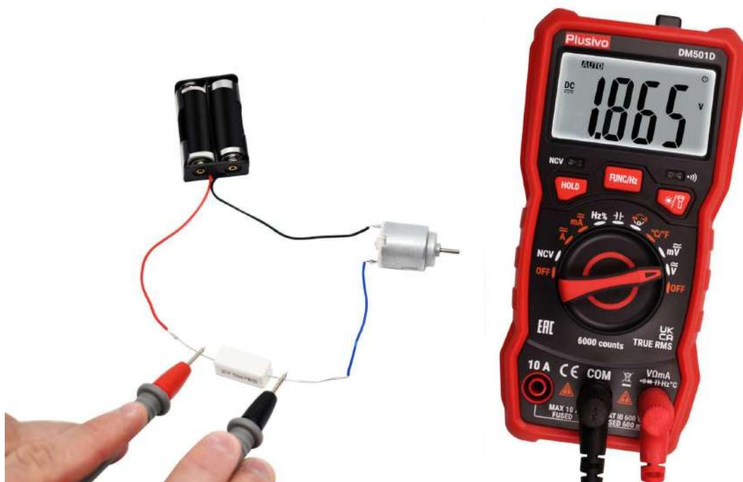
The measured voltage in this figure is 1.865 V DC.
