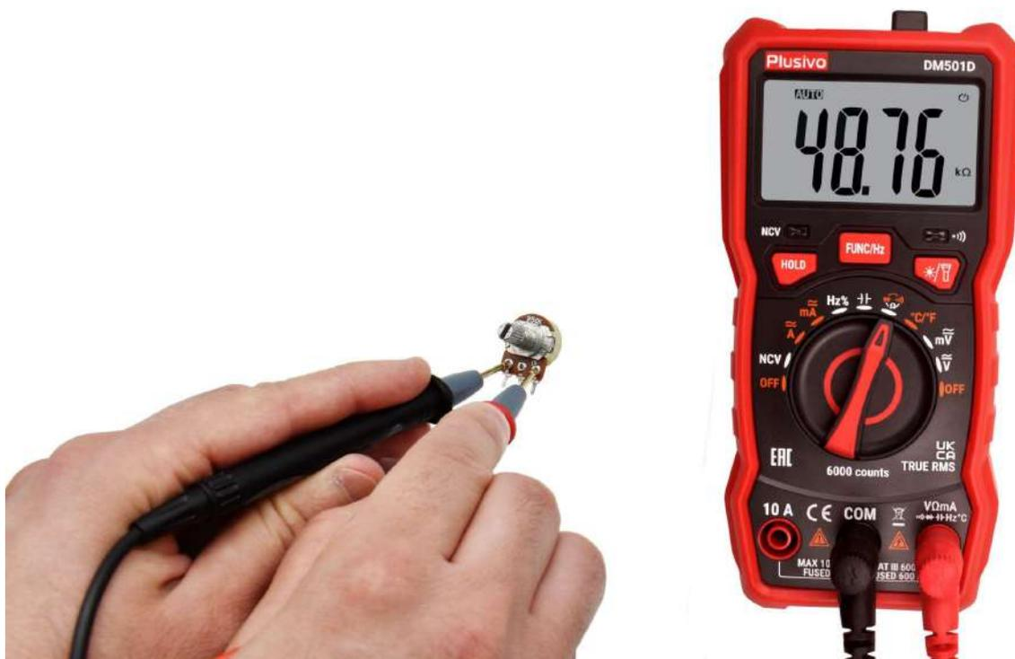
**The measured resistance in this figure is 48.76 kΩ.**
