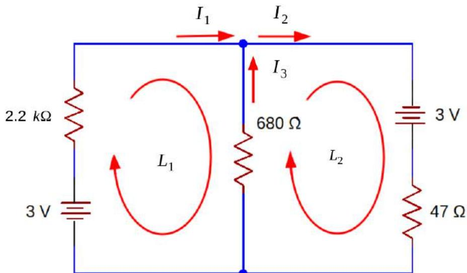
The equation  $I_1 = I_2 + I_3$  will be changed to:  $I_2 = I_1 + I_3$
