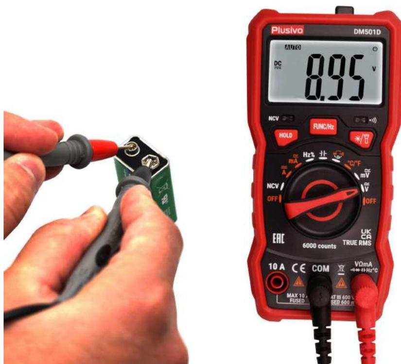
The measured voltage in this figure is 8.95 V DC.
