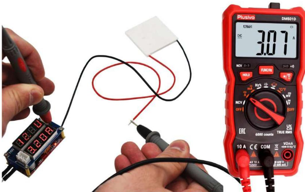
In this set-up, the red probe is inserted in the 10A socket for DC current setting. The reading is 3.07 A.
