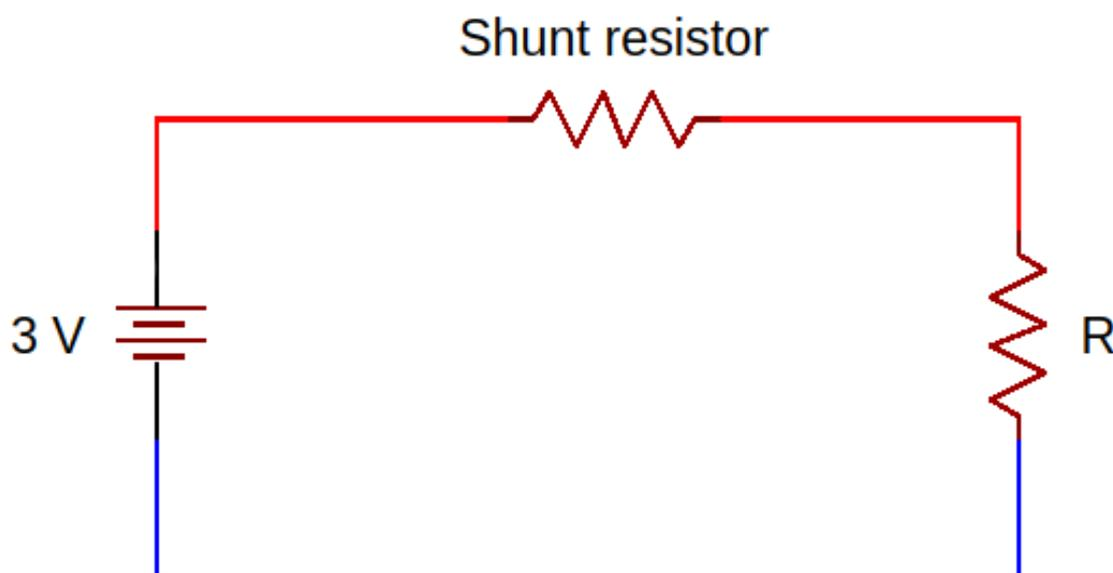
So depending on ohm's law " $V = I \cdot R$ ", we have a shunt resistor, and we have a current passing through it, so the voltage will be generated around it. And then we will measure this voltage using the multimeter, this way we have converted the current into voltage.
