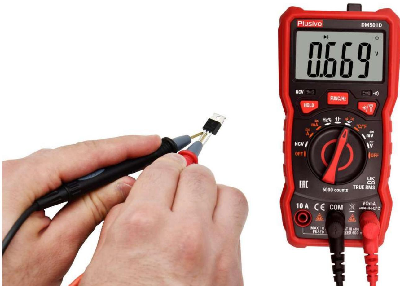
The measured forward voltage is 0.669 V.
