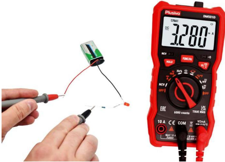
The measured current in this figure is 3.280 mA.
