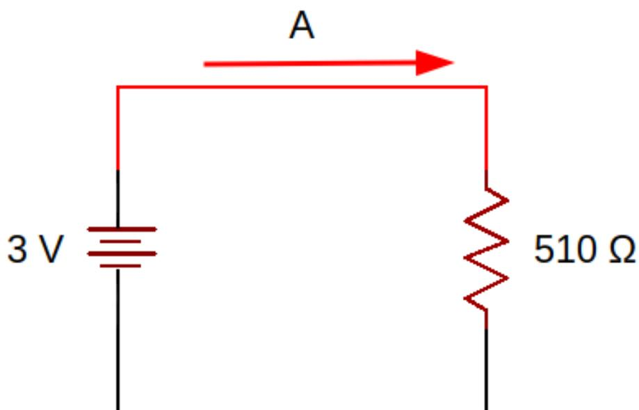
To calculate the power on the resistor, we need any two values of these: **Voltage**, **Current** or **Resistance**.
