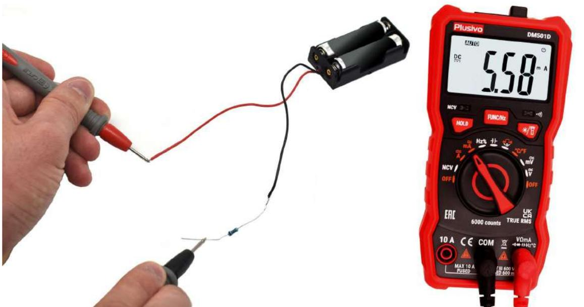
But indeed, we can count on our calculation " $3 \text{ V} / 510 \Omega = 5.88 \text{ mA}$ " because 5.88 mA is almost equal to 5.61 mA.
