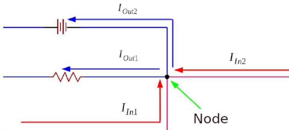
$$I_{In1} + I_{In2} = I_{Out1} + I_{Out2}$$
