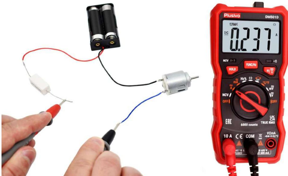
The measured current in this figure is 237 mA.
