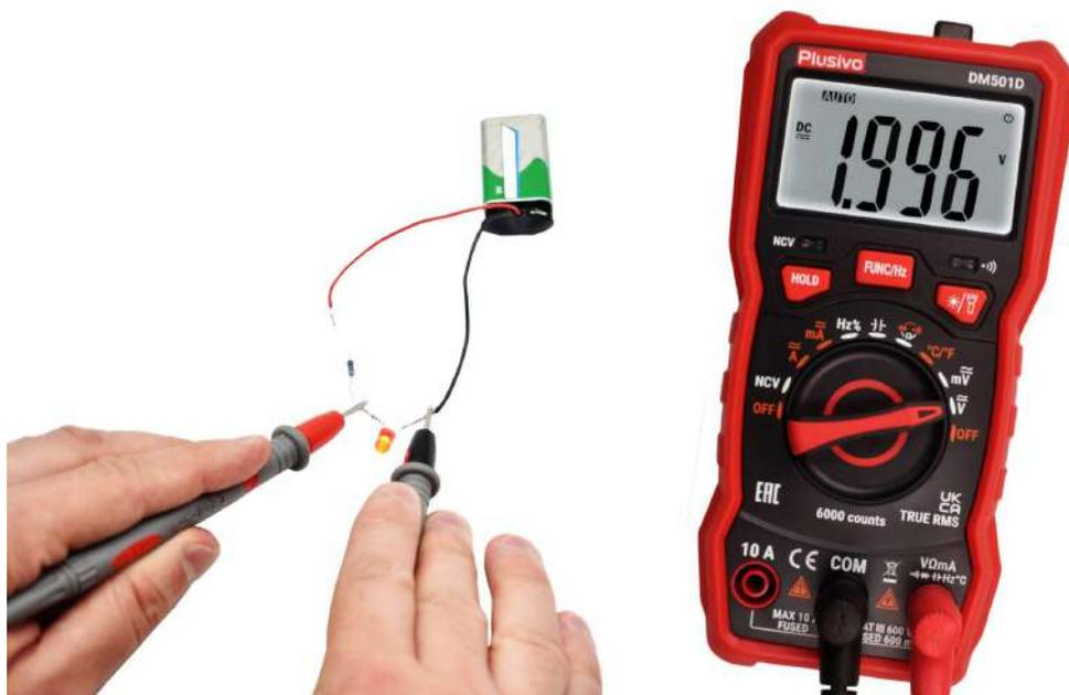
The measured voltage in this figure is 1.996 V DC
