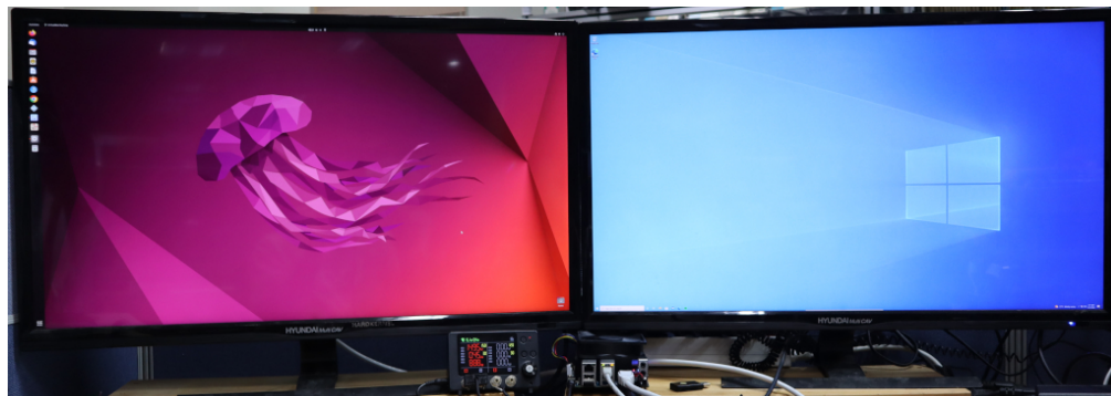
Picture 2 : The monitor on the left shows Ubuntu Desktop host OS and the one on the right shows Windows 10 running as a guest OS, using the hardware virtualization VT-x technology.
