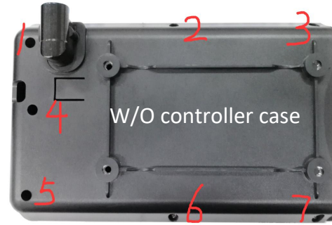
3. Close the upper and lower cover with 7 ST2.9*10 round head cross screw.
