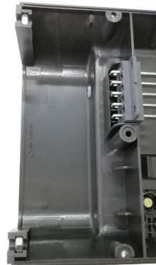
3. Snap 2 M5 nuts into the controller case.
