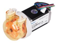
Two kinds of stepper motor: 12V / 24V Flow rate range: 11.5ml/min ~ 71.5ml/min Working conditions: temperature 0 ~ 40 ° C, humidity < 80% Pump tube selection: silicone tube, Pharmed? BPT tube Pulsation: 3 rollers, moderate pulsation Pump head: engineering plastics Weight: 225 g
