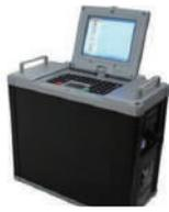
On-line flue gas detector
