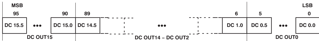
Figure 14. Dot Correction Data Packet Format
