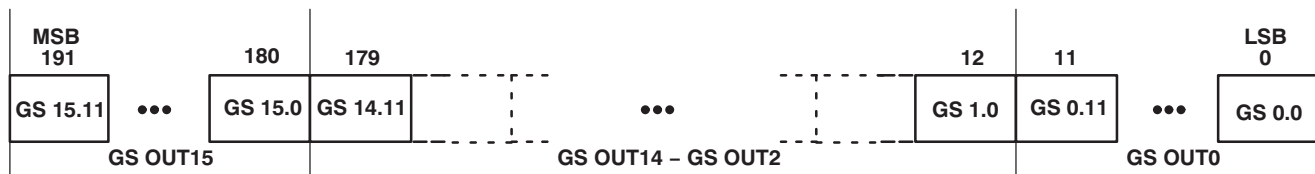
Figure 18. Grayscale Data Packet Format
