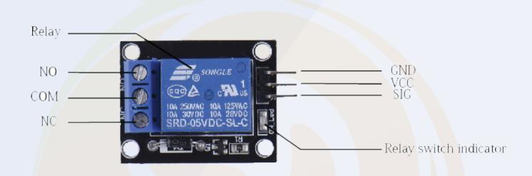
In the above image you can see COM, NC and NO pins. These are connected to the load.
