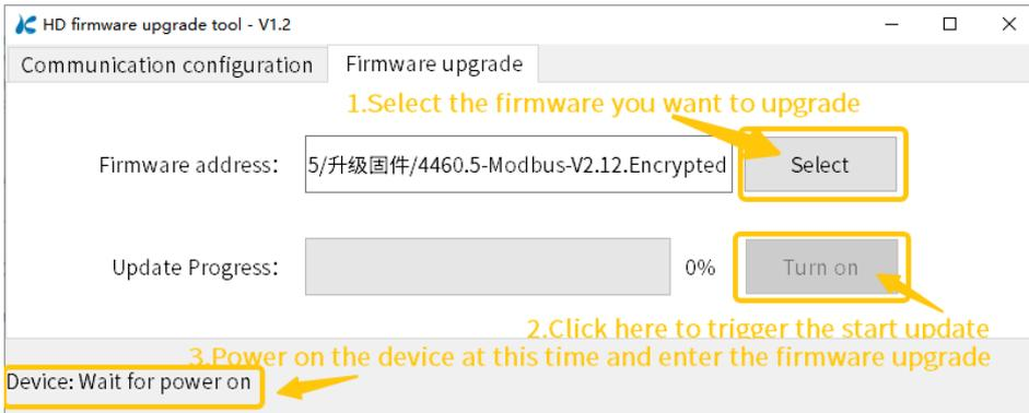
(5) After waiting for about 2 minutes, the firmware upgrade can be completed. After the upgrade is completed, the update progress is displayed as "100%". At this time, you can close the firmware upgrade tool and use it normally.
