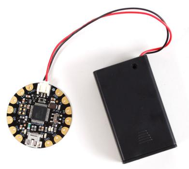
After loading your program onto the FLORA, you'll want to unplug the USB cable and go portable with battery power! USB will always power the board, but battery power (through the JST connector) can be turned on and off with Flora's onboard switch (near the "ON" text on the board). We recommend our 3xAAA holder (http://adafru.it/727) for beginners, which conveniently plugs into FLORAs JST port.
