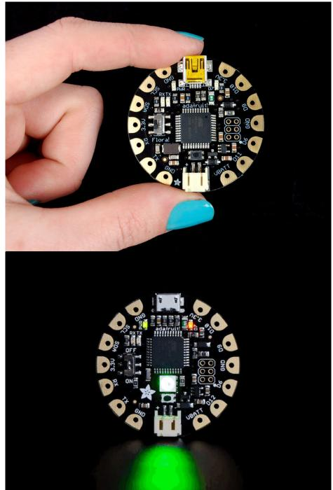
FLORA is Adafruit's wearable electronics platform. We designed it from the ground up to provide the best experience for Adafruit's community of makers, hackers, crafters, artists, designers and engineers. It's built around the Atmega32u4 chip, which has built-in USB support. No pesky special cables or extra parts for programming, just plug it in and get started making the wearables project of your dreams! Works on Windows and Mac.
