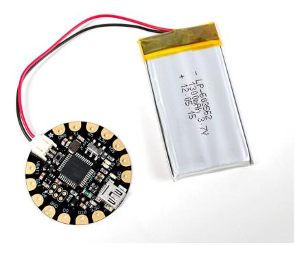
More advanced users may wish to use a rechargeable lithium polymer battery (http://adafru.it/258) for their smaller size and longer duration. These batteries pose added risk if abused, shorted, bent, crushed, or punctured. FLORA does not have onboard charging, so you would also need a separate LiPoly charger (http://adafru.it/259).
