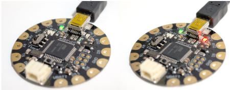
That's it! The on board LED marked "D7" should blink on and off repeatedly, and you've successfully programmed your FLORA!
