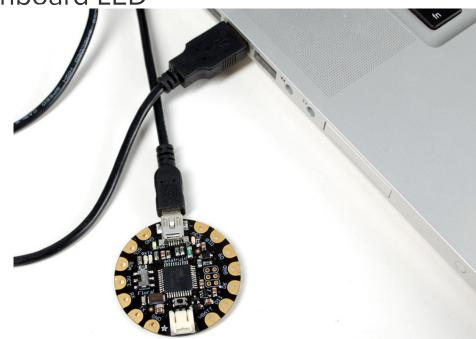
Next it's time to load up a program on your FLORA. There is an LED on board, so let's blink it! Plug in the USB cable and paste the following code into the Adafruit Flora IDE:
