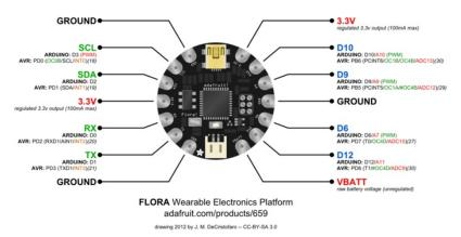
For handy reference, we've created this pinout diagram illustrating all the alternate functions for each of the pins on the Flora.
